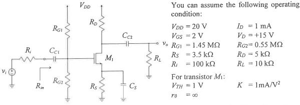
Note: you can ignore the high frequency equivalent circuit model for  $M_1$ . (i.e.  $C_{gs1} = C_{gd1} = 0$ )
