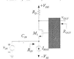
a) Determine the input and output resistance ( $R_{IN}$  and  $R_{OUT}$ ) if there is no feedback network (i.e.  $R_1 = \infty$ , and  $R_2 = 0$   $\Omega$ ).
