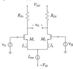
This differential amplifier uses a bias current of  $I_{bias} = 20 \mu A$
