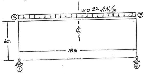
Use the moment-distribution method to analyze the structure shown. Draw shear and bending moment diagrams. On both diagrams, for each member, label the magnitudes of maximum and minimum ordinates (Minimum ordinates are frequently negative values). All members have the same EI value and are inextensible.
