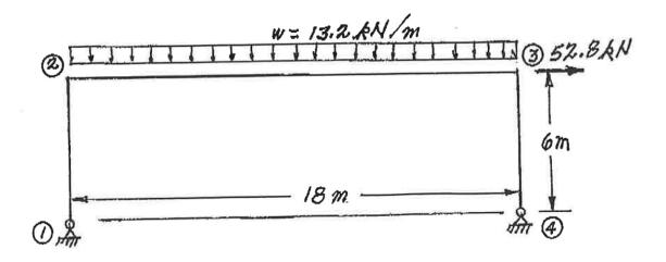
(22) 8. Using the slope-defection method or the moment-distribution method, analyze the frame structure shown below. Plot shear force and bending moment diagrams. For both diagrams, on each member label the magnitude of the maximum and minimum ordinates (Minimum ordinates are frequently negative values). All members are inextensible and have the relative EI values shown. Take advantage of symmetry.
