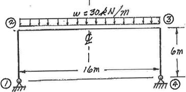
Using a flexibility (force) method, analyze the frame structure shown. All members have the same EI value and are inextensible. Draw shear and bending moment diagrams. On both diagrams, for each member, indicate the magnitudes of the maximum and minimum ordinates (Minimum ordinates are frequently negative values.).
